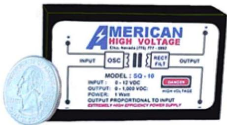
The SQ Series is a line of compact high voltage DC to DC converters that have been designed especially for battery operated systems where high efficiency is required. Like their SC cousins, the SQ models are rugged, arc resistant, and virtually burn-out proof. Power transfer efficiencies up to 80% are standard as is seen by the very low input current required for operation. The output power of all SQ models is limited to 1.5 Watts. All SQ's are reverse input voltage and short circuit protected.
